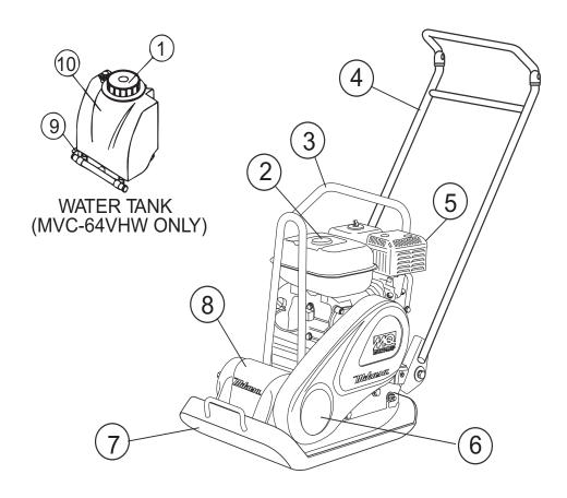
Figure 3. MVC-64VH/VHW Plate Compactor Components
